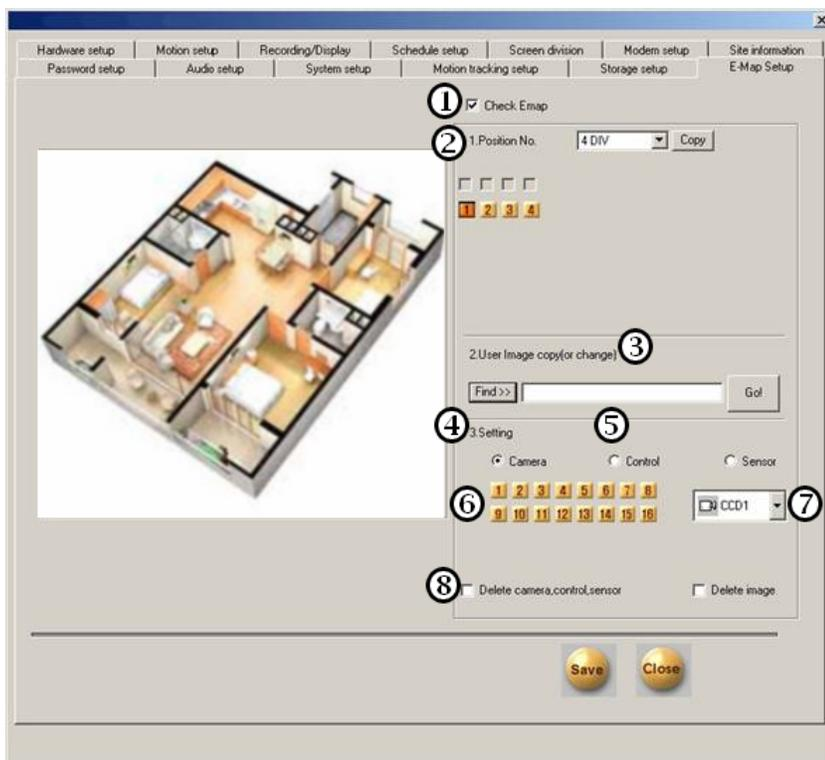
*E-Map tab contains the settings for EMap. EMap is a computer map of area with designated locations of installed cameras, sensors and controls.*
