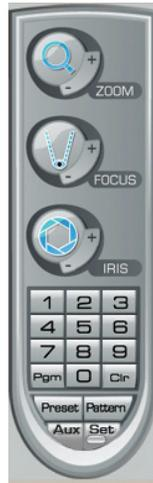
**Figure 66.** PTZ Control Toolbar with Camera Lens Controls
