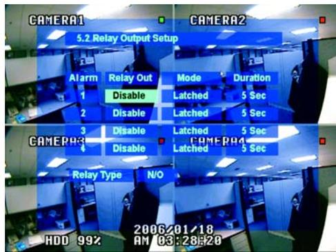
**Figure 38.** Relay Output Setup Menu
