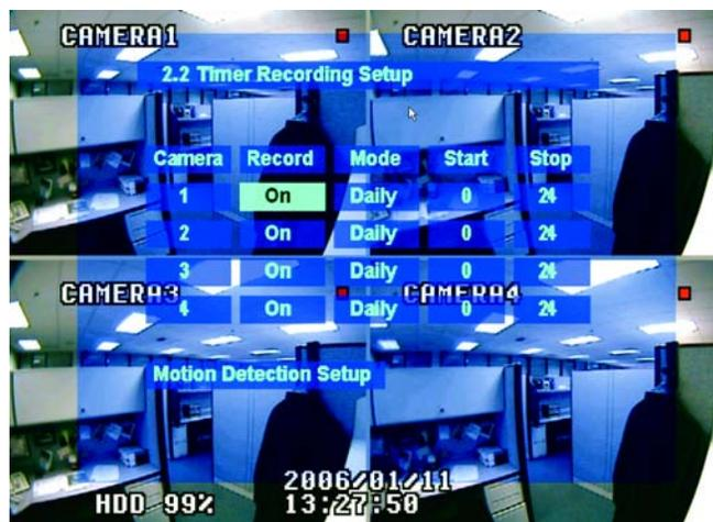
Figure 40. Timer Recording Setup Menu
