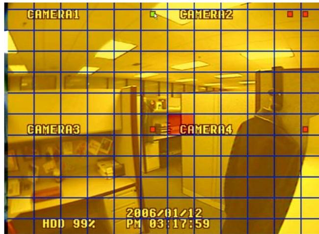
**Figure 45.** Motion Detection Region Setup Screen
