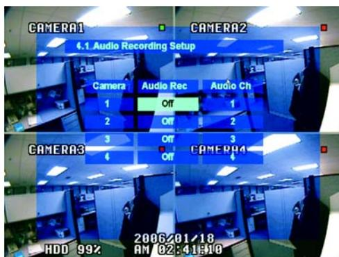
**Figure 33. Audio Recording Setup Menu**
